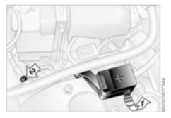
The auxiliary jump-starting terminal located in your BMW's engine compartment acts as the positive battery terminal. The cover of this auxiliary terminal is marked with a + sign. Remove by pulling the tab - see arrow 1.
